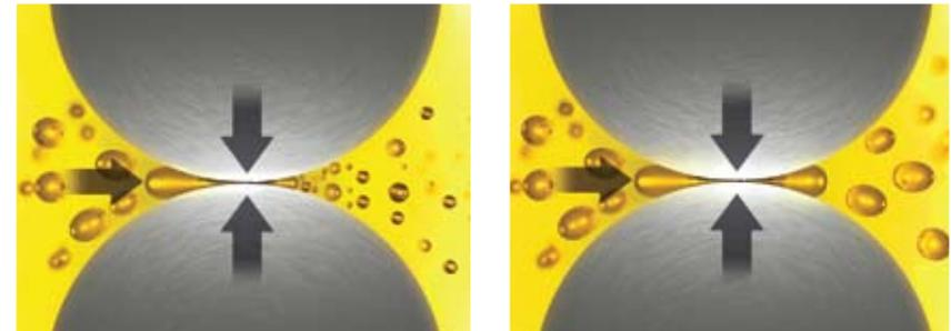
**SOME OILS:** Large molecules can be torn apart by shearing forces. The oil’s viscosity is reduced, and engine friction and wear can increase if the oil film gets too thin.
